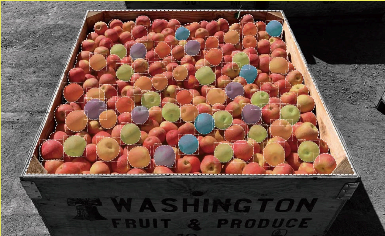
The Spectre for Apples computer vision fruit-sizing tool begins detecting apples from the top of the bin
